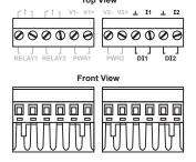
STEP 1: Insert the negative (ground)/positive DI wires into the \(^1/11\) terminals
