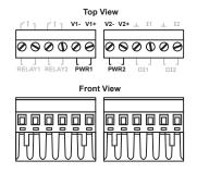
**STEP 1**: Insert the negative/positive DC wires into the V-/V+ terminals.
